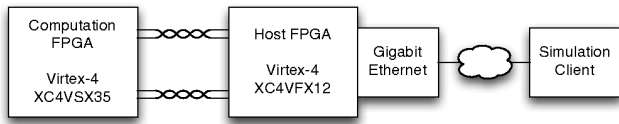
Fig. 3. The computation FPGA is a Xilinx Virtex-4 XC4VVSX35 FPGA. The host FPGA is a Xilinx Virtex-4 XC4VFX12 FPGA, incorporating a PowerPC 405 core and a Gigabit Ethernet interface. The two FPGAs are interconnected via a 2 Gbps proprietary interface.
