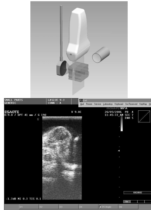
Fig. 1. Left: Configuration of the integrated imaging/HIFU system showing the intersection of the imaging plane with the HIFU focus. Right: A screen capture showing a B-mode image of the tumor in the hind limb of a nude mouse.
