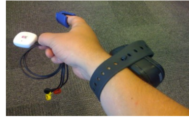
Fig. 2. Telemetry-based vital-sign sensors. The Bluetooth relay band is connected to the \text{SpO}_2 sensor and transmits the pulse-oximetry signal to the PDA
