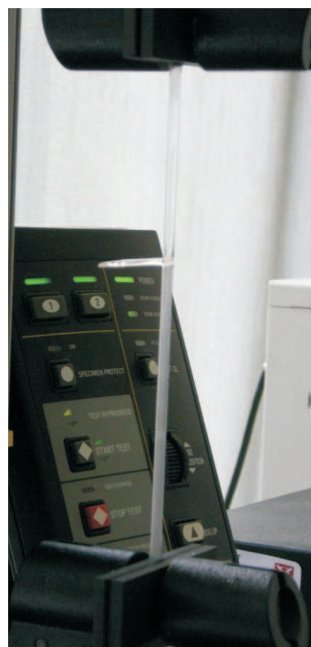
Fig. 8. The force was measured to peel the two silicone layers from each other with a pulling machine.
