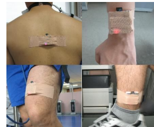
Fig. 2. Locations and Directions of Triaxial Accelerometer Attachment
