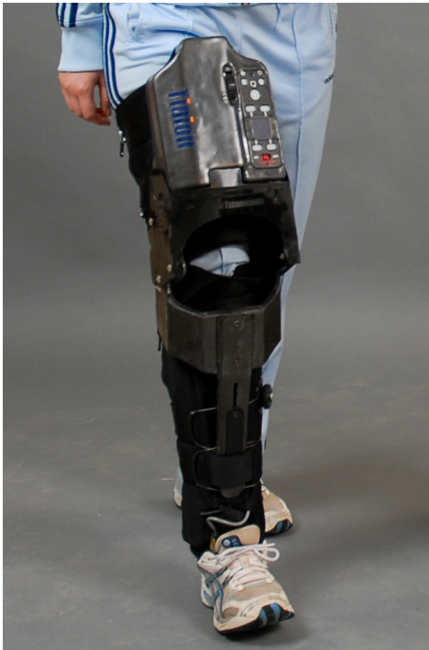
Fig. 1. The Tibion® PK100 bionic leg orthosis
