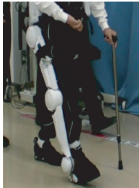
Fig. 4. Single leg version of the HAL fitted to the subject
