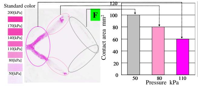
Fig.7 The result of the pressure distribution
