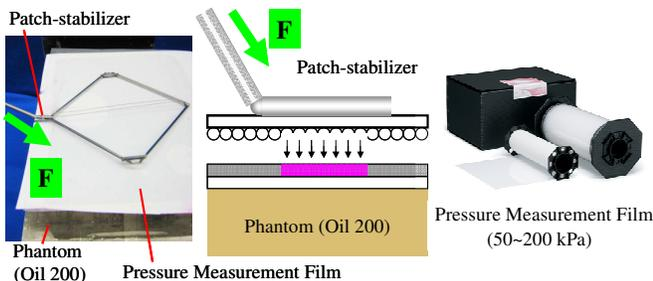
Fig.6 The measurement system of pressure distribution
