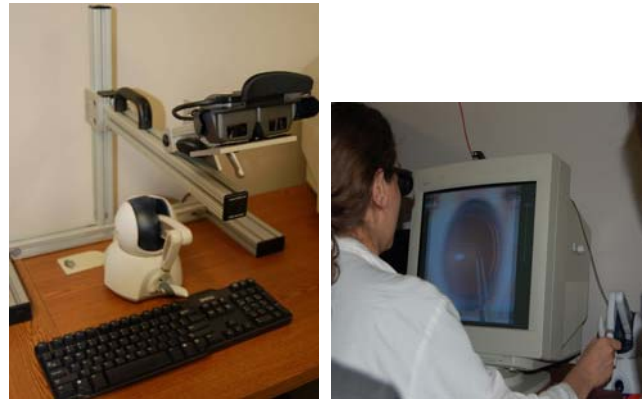
Fig 2. HMD (left) version and CRT monitor (right) version of the system
