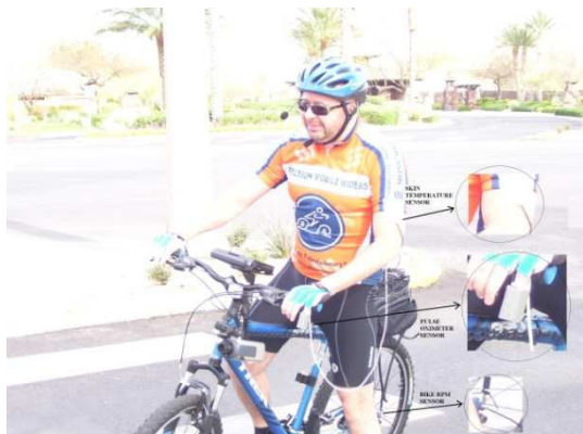
Fig. 4. Bicycle RMMS showing the various sensors connected to the rider.
