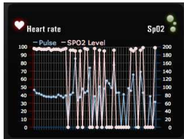
Fig. 3. Bicycle Rider Heart Rate and SpO 2 . The reason for the zero values for heart rate and SpO 2 is where the sensor does not detect a finger in the device, caused by either too much outside light interfering with the sensor LED or sweat on the finger is interfering with the sensor LED.
