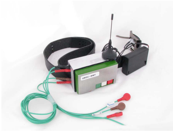
Fig. 2. Wearable Biomedical Signal Measurement Terminal (Package).
