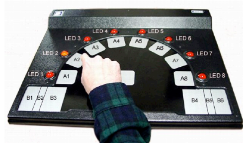
Fig. 5. The BEP I Central Processing and Upper Extremity Motor Control Performance Capacity Measurement System.
