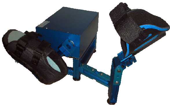
Fig. 1. Intelligent ankle stretching device. The device can be configured to treat either left or right ankle. The size of the footplate and the position of the leg support can also be adjusted.
