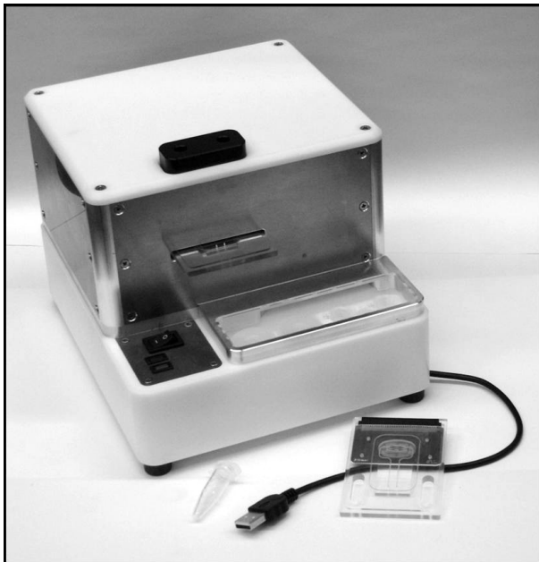
Fig. 2. The latest version of NRL's shoebox sized compact Bead Array Sensor System ( cBASS ® ). It is a fully automated device with integrated signal processing electronics and microfluidic actuation system. Assays are performed on the BARC ® chip mounted in a microfluidics cartridge.
