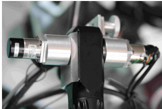
Fig. 9. Motorization of the arms
