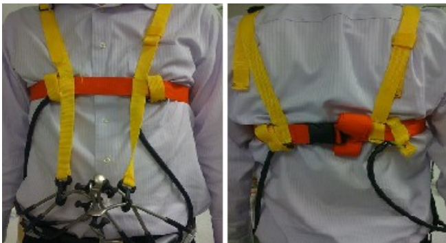
Figure 2 – Anterior and Posterior Views of the Electronic Stethoscope Array Harness Embedded with 4 Stethoscopes Attached to a Human Torso
