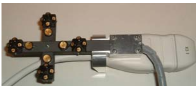
Fig. 6. Tracking the 3D echo probe by using the Optotrak system.
