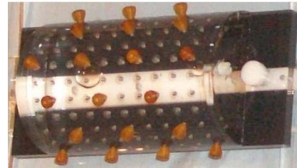
Fig. 3. The X-ray system calibration phantom
