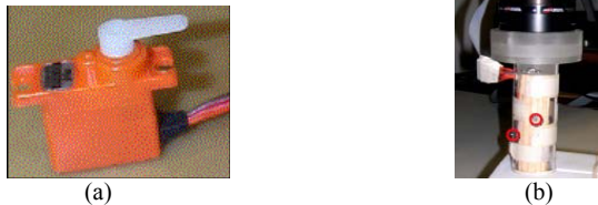
Figure 2. (a) A servo motor; and (b) four small servo motors mounted on cuboids inside a plastic handle.
