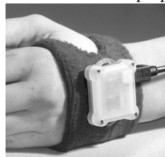
Fig. 3. Triaxial accelerometer enclosed in sealed case and attached on the dorsum of the hand.
