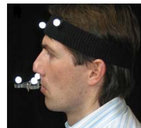
Fig. 3 6 DOF motion capturing using a special paraocclusal framework attached to the lower set of teeth to record mandibular movements and a headband with three retro-reflective markers to record cranium movements
