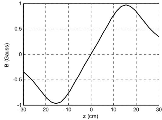
Fig. 2. A simulation result showing relationship between location and magnetic field by a Maxwell coil ( $h=2r=30\text{cm}$ ).
