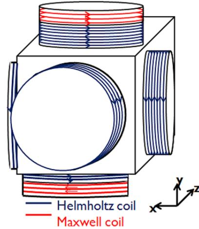
Fig. 1. The coil system consisting of three orthogonal Helmholtz coils and a Maxwell coil. The heights of the coils have been changed to fit on the cubic surface.
