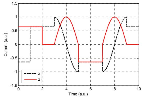
Fig. 5. An example of a desired navigation path (top) and corresponding Helmholtz coil current waveforms (bottom).
