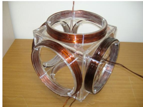
Fig. 3. The fabricated coil set consisting of three Helmholtz coils and a Maxwell gradient coil.
