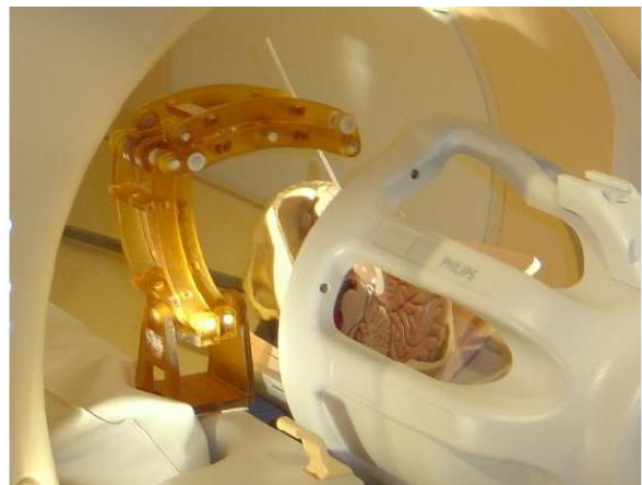
Fig. 1. The prototype robot in the bore of a 3T MRI scanner with the cannula targeting a model skull.
