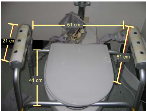
Fig. 1. Commode grab bars instrumented with embedded pressure sensors
