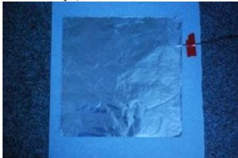
Figure 1 Aluminum foil covered by vinyl (for protection and ease of use) with leads glued in place.
