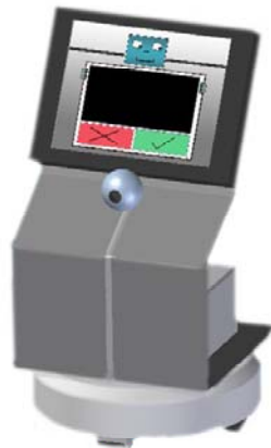
Fig. 1. Conceptual rendering of the SKOTEE home robot system. The current prototype is based on the iRobot Create® development platform.
