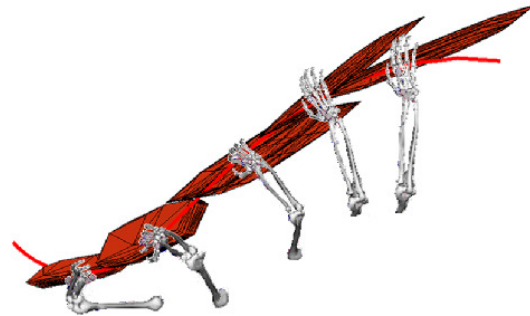
Fig. 5. The feasible set of accelerations for selected 5 configurations of a throwing motion. The throwing hand follows the direction defined by the maximum acceleration at each configuration [6].
