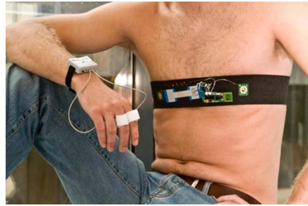
FIG. 3. Integrated body area network for ambulatory monitoring of physiological responses from the Autonomic Nervous System
