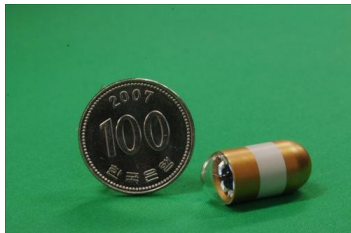
Figure 1. Miniature video capsule by Given Imaging[1]
