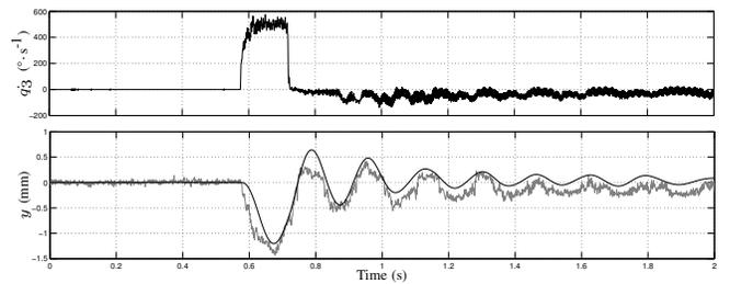
Fig. 5. On top the window control imposed to the system input. On bottom the output response comparison between experimental system (gray) and identified model (black).
