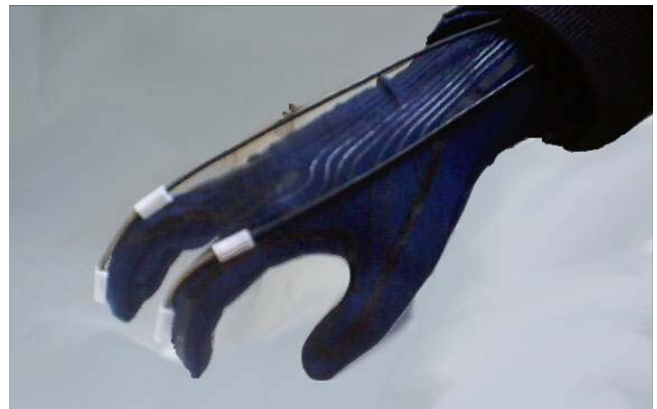
Figure 3. Worn sensorized glove during a testing phase in comparison with commercial electrogoniometers
