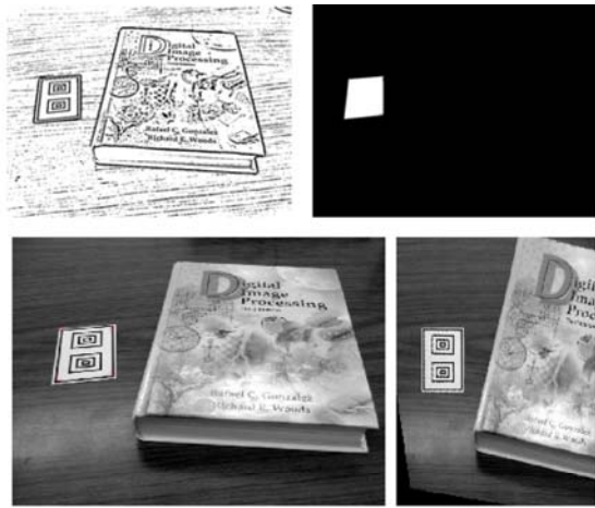
Fig.2. Corner detection and perspective correction. In raster scan order: Binary image after adaptive thresholding; Detected reference card; Corners of the card are marked on the image; Perspective correction of the card.
