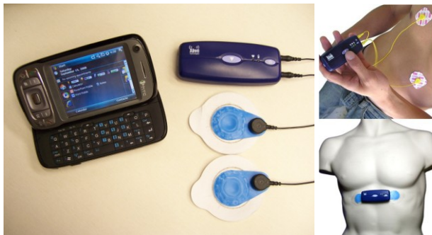
Fig. 2. HeartToGo Prototype, including an HTC PDA phone with Microsoft Windows Mobile 6 and a single channel Alive Heart Monitor. Two standard lead configurations: [Upper-right] chest leads with wire connection; [Lower-right] chest leads with snap connectors [1].
