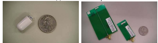
(b) Capsule-sized signal generator and antennas (left: for except 2450 MHz, right: for 2450 MHz) used in the measurements.
