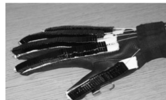
Fig.1. Structure of the J-Glove. Cables run through chains of cable guides.
