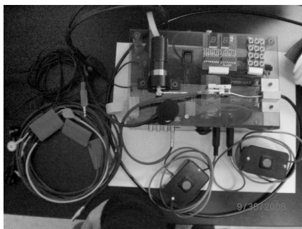
Fig.6. Picture of the Final prototype. It shows the electronics components: Motor, tension sensor, buttons, EMG circuits, microphone.
