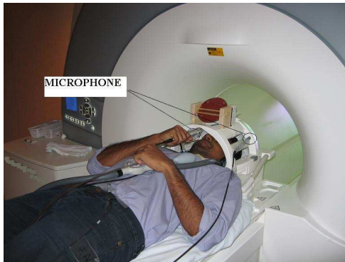
Fig. 4. Real fMRI experiment used to record speech plus noise with a Siemens 3-Tesla MRI system. The targeted application is speech enhancement during fMRI experiment. N = 2 .
