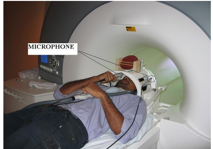
Fig. 1. Speech Enhancement setup on an MRI machine. The picture shows two microphones. The primary microphone is held by the subject and the reference is connected to the head matrix. The microphones are kept from 15 to 20 cm apart.
