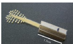
Fig. 3. The multi-channel arrayed polyimide based electrode
