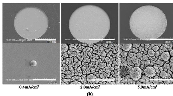
Fig. 4. (a) electro-plated surface with conditions, respectively. (b) SEM image of method #02 by electro-plating 0.4 mA/cm<sup>2</sup>, 2.0 mA/cm<sup>2</sup>, 5.9 mA/cm<sup>2</sup>.
