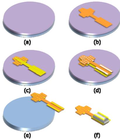
Fig. 1. A schematic overview of polyimide based electrode process. (a) Sacrificial layer (Al). (b) Polyimide for 1<sup>st</sup> layer spin-coating and patterning. (c) Metallization (Ti/Au). (d) Polyimide for 2<sup>nd</sup> layer spin-coating and patterning. (e) peel-off the polyimide base electrode. (f) Connector connection.
