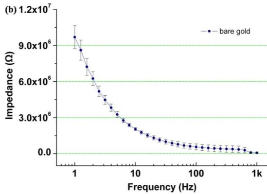
Fig. 5. (a) measured the impedance of electrode electroplated with method #02. (b) measured the impedance of bare gold, non-electroplated on seed layer.
