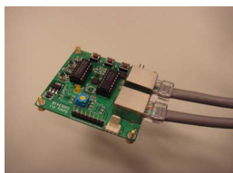
Fig. 8. Fail-safe interface prototype board
