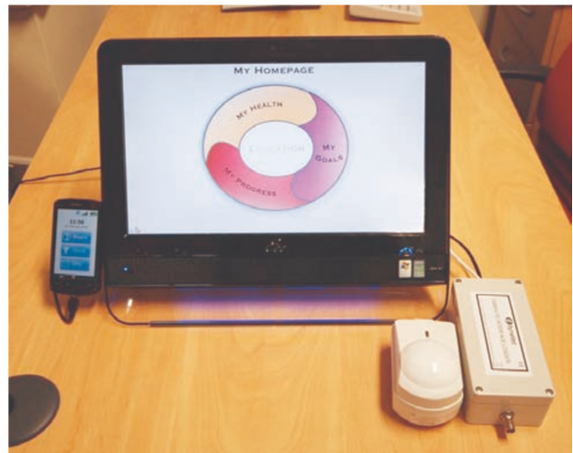
Figure 4. CHF PSMS deployed for user evaluation. The system included the mobile device and telehealth devices.
