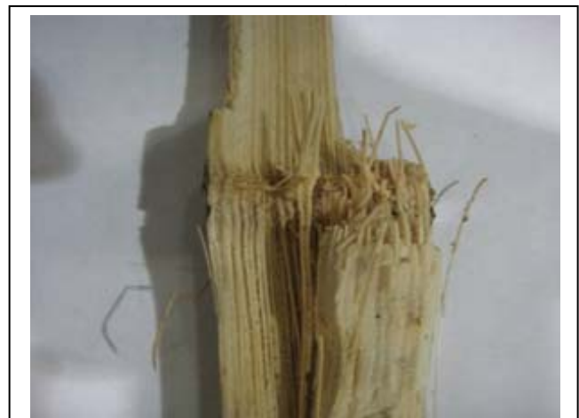
Fig. 1. Vascular bundles in a fragment of corn stover. Cellulose fibrils are arranged approximately parallel to the long axis of vascular bundles. Centimeter-long segments of approximately two dozen vascular bundles were arranged along the surface of a copper cold finger through which liquid Nitrogen was circulated. A Beryllium dome was used to cover the sample which was evacuated in order to prevent the build-up of ice crystals on the sample.
