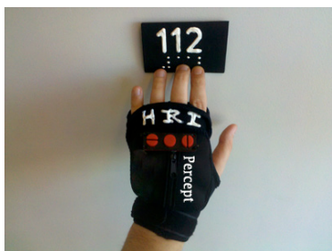
Figure 2. PERCEPT Glove (back view) Scanning an R-Tag
