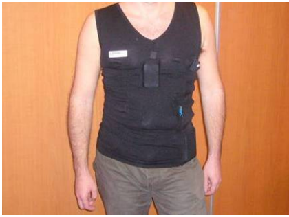
Fig. 2. The wearable platform with all sensors integrated to the CHRONIOUS jacket
