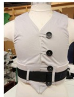
Fig. 5. Bio-impedance sensor embedded in the HF vest.
