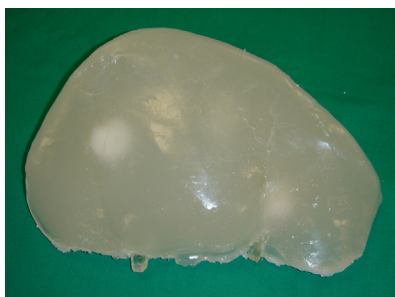
Fig. 2. Phantom appearance: cellulose decreases candle gel transparency and constitutes echogenicity, agarose tumors are visible inside of the phantom.
