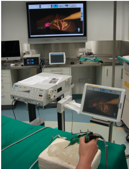
Fig. 6. Experiment: touching of tumor models in the liver phantom with registered instrument. A test person was only allowed to use the display (on the top) while puncturing the tumor models in the phantom (on the bottom) with the instrument tip.
