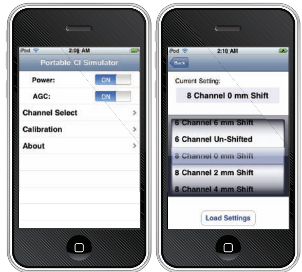
Fig. 2. Graphical user interface for a portable cochlear implant simulator. The screen on the left shows the default view when starting the program. The screen on the right allows for specification of the channel and basalward shift.
