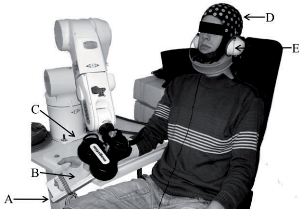
Fig. 1. Measurement setup for the peripheral magnetic stimulation using the TMS system. A - non-conductive fixation, B - arm cover, C - figure-8 stimulation coil, D - 128 channel EEG cap, E - ear protection
