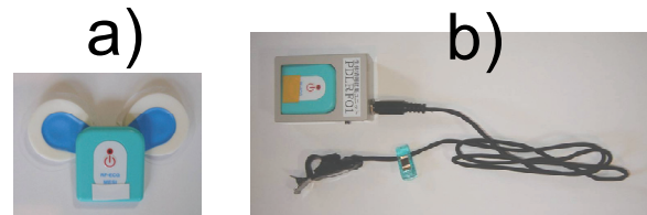
Fig. 1 Wireless sensors for measuring a) ECG signal and b) photo-plethysmographic signal
