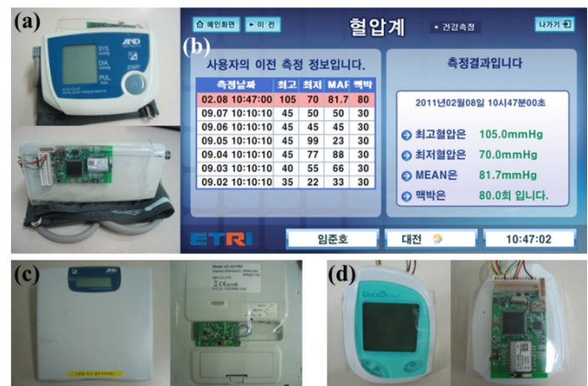
Fig. 7. Standardization of 3 healthcare devices using the proposed toolkit: (a) is a blood pressure monitor standardization, (b) is a measurement GUI result of the home health gateway, (c) is a weight scale standardization, and (d) is a glucose meter standardization.
