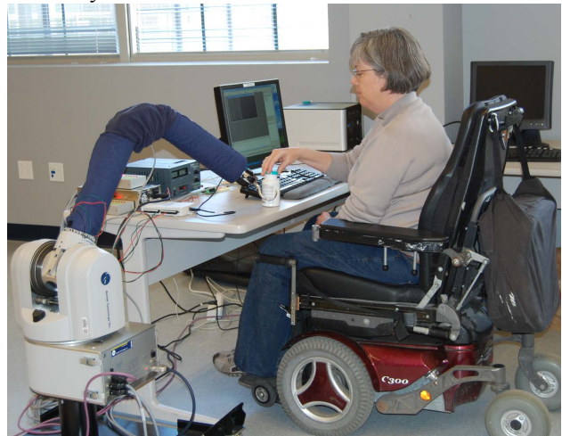
Figure 1. A prototype system for investigating direct interaction with an assistive robotic arm. When the individual grasps the touch-sensitive skin, the robot moves compliantly. When the skin is released, the robot remains fixed in position.
