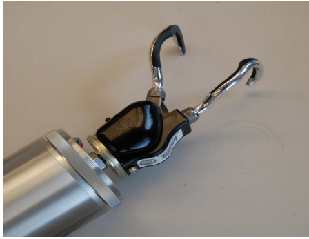
Figure 3. The prehensor used in this system, the Electric Terminal Device (ETD) from Motion Control.
