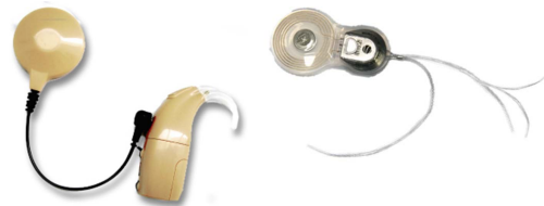
Fig. 2. An integrated vestibular-cochlear implant system with additional leads for semicircular canal stimulation
